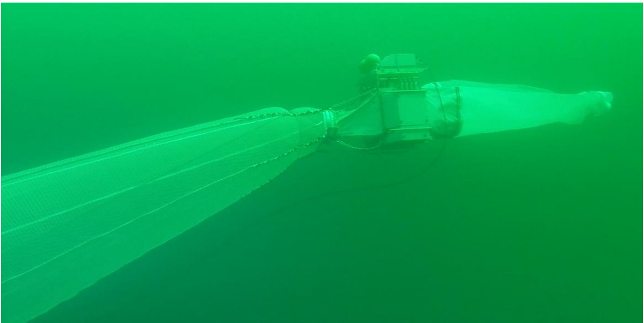
Figure 8: The MultiNet attached to the IKMT at a depth of approx. 30 m (Foto: A. Hermann)
