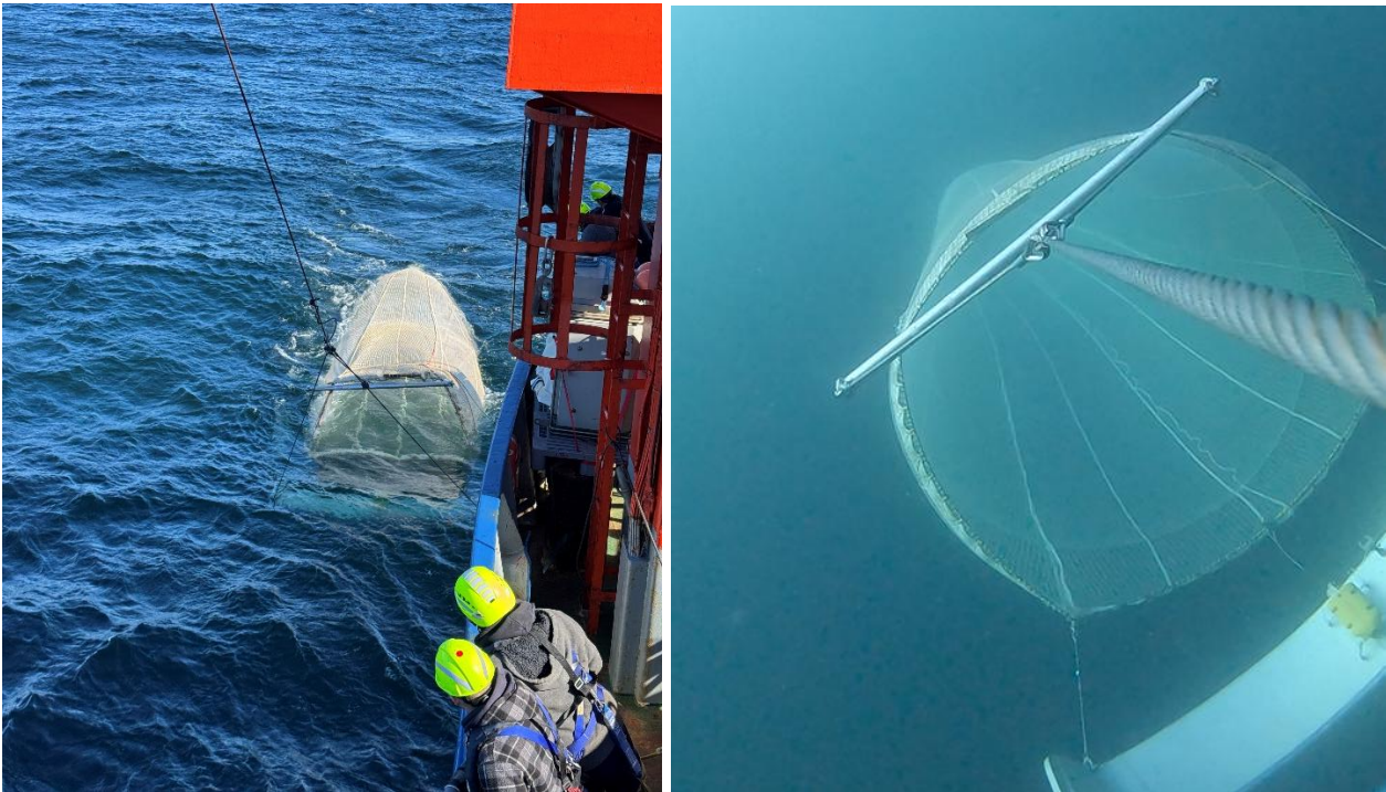
Figure 7: Deployment of the IKMT (left, D. Stepputtis) and view into IKMT net opening (right, L. Marohn)
