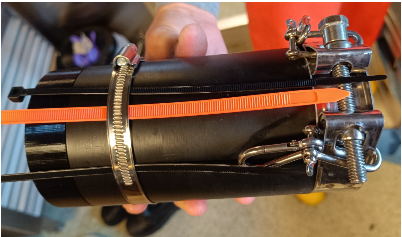
Figure 3.5.3. Cod end sampler ready for the attachment to the trawl net with cable ties, hose clamps and carabines.
