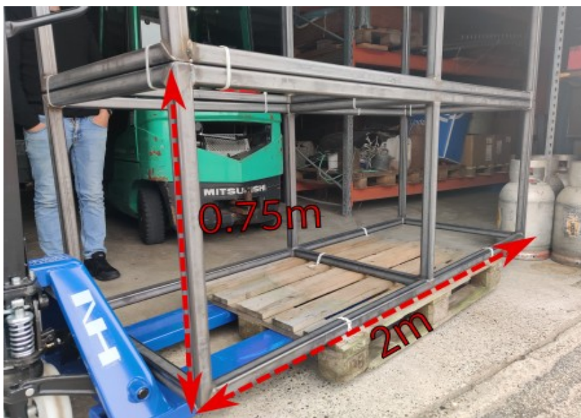
Figure 1: Rigid frames (two units stacked) used to fix the mesh geometry at OA = 40°, 60° and 90°.
