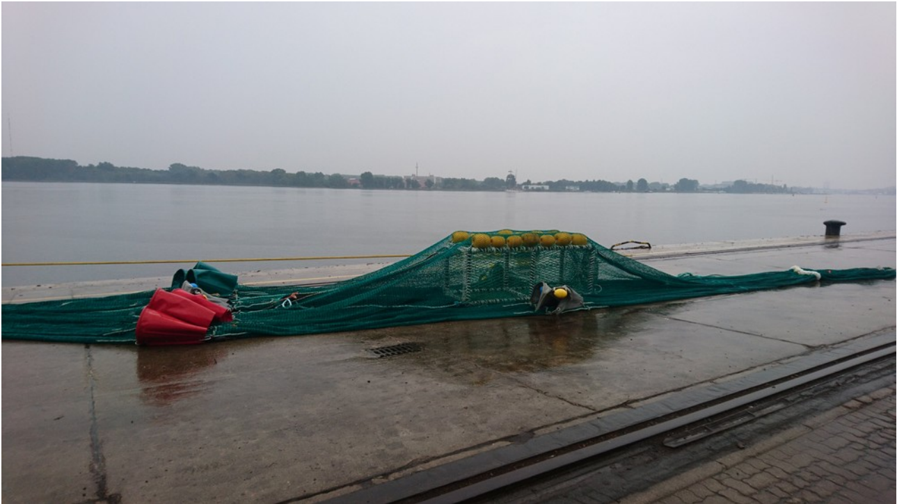
Figure 3: Lateral view of the experimental OA40 codend surrounded by the cover. The cover was rigged with forward (red, green and grey) and lateral kites aligned to the mid-length of the codend (grey). To compensate for the negative buoyancy of the OA40 codend, the device was initially rigged with 2x floating lines consisting of 7x foam buoys that were attached side by side along the longitudinal upper bars of the frame.
