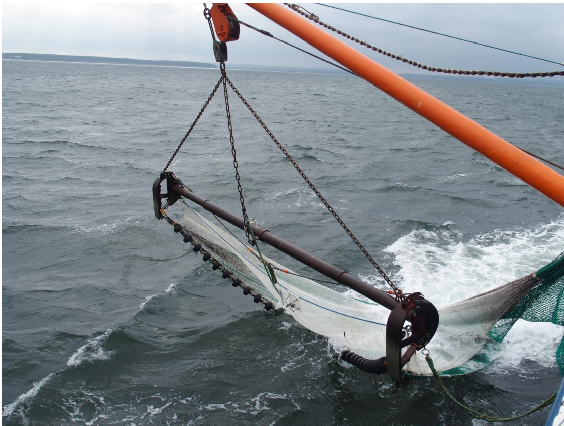
Abbildung 27: Schlepp-Hahnepot am Kurrbaum Figure 27: towing bridles on the trawl beam
