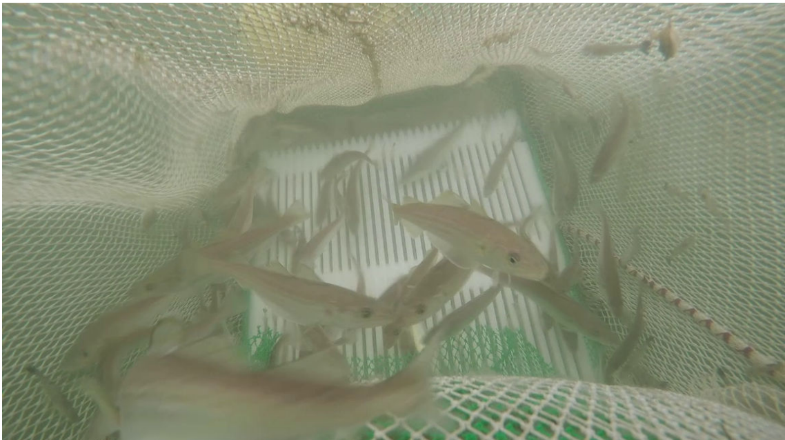
Figure 22: Whiting swimming in front of the Single-grid gear design 6. the net at the bottom of the image correspond to the guide panel covered with 16 mm netting (green meshes). The camera position can be checked in Figure 10
