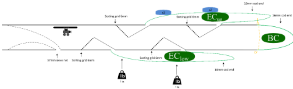
Figure 17: Details of Multi-grid gear design MG3
