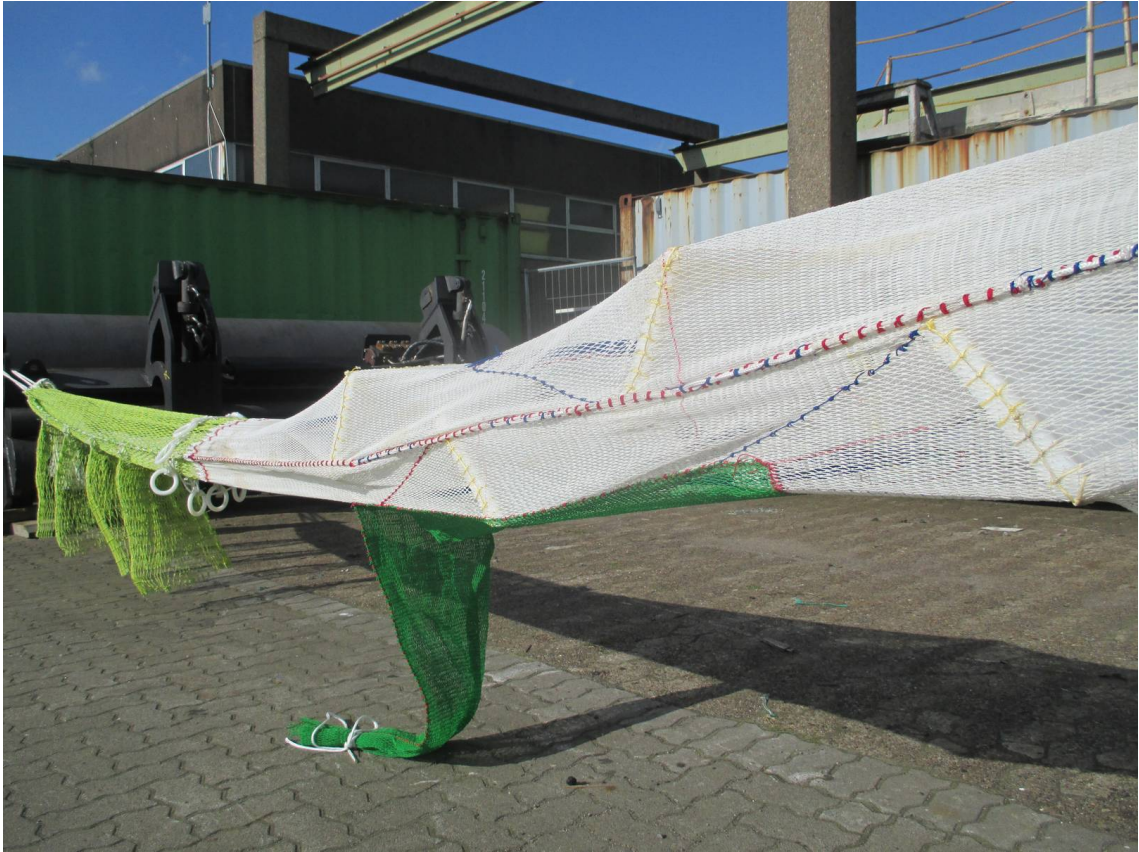
Figure 4: Multi-grid gear under construction in the net loft.
