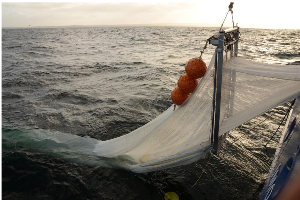
Figure 2: Multisampler for pelagic trawls (here: PSN Krake) during test at SO715
