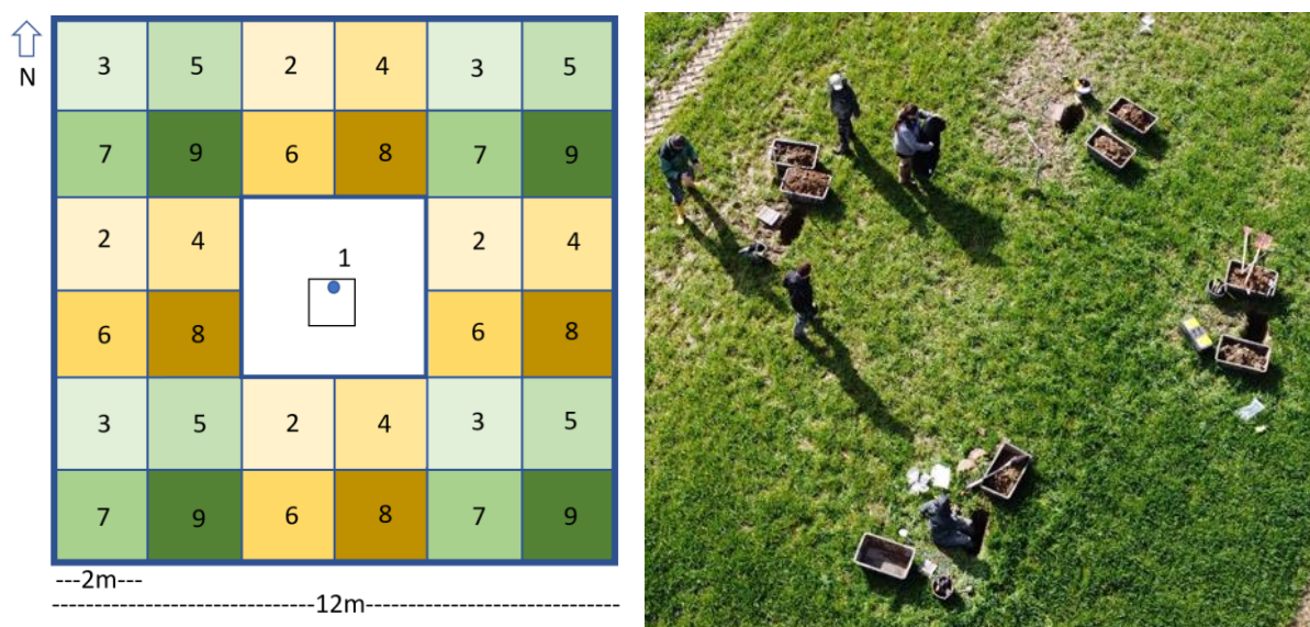
Figure 1 Sampling scheme for up to eight repeat inventories (marked by numbers 2–9) and drone image of a joint sampling of a site with four simultaneously opened profile pits. No. 1 marks the location of the central soil profile of the initial BZE-LW.
