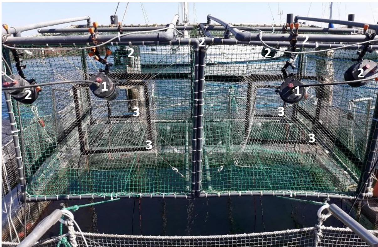
Fig. A4. Experimental pot with two exchangeable entrances. Two IR cameras (1) in front of each funnel entrance and two IR lights (2) on each entrance side (one inside above the funnel inner opening, the other outside next to the IR cameras). Black frames around funnels are RFID antennae (3). Note: Owing to technical difficulties, RFID data could not be used in the data analysis.
