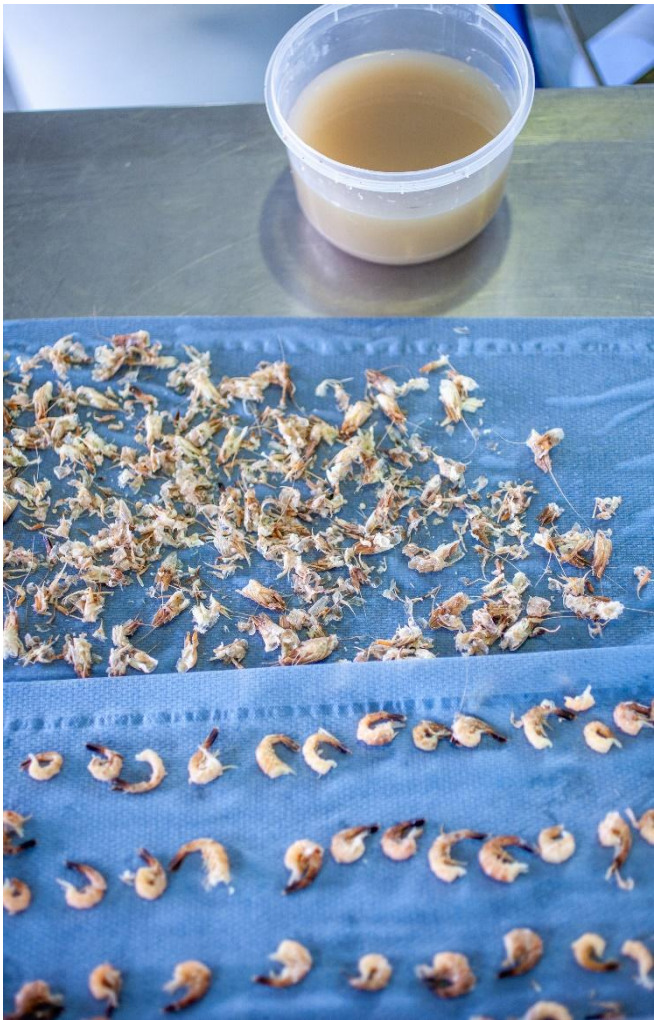
Figure 3: The three products ("streams") from mechanical de-shelling. From bottom to top: shrimp meat (freed from its shell, here still with the shell fragments - darker in color - detached but not yet shed at the tail end), shell remains. and process water (©Thünen Institute/H. Brückner)
