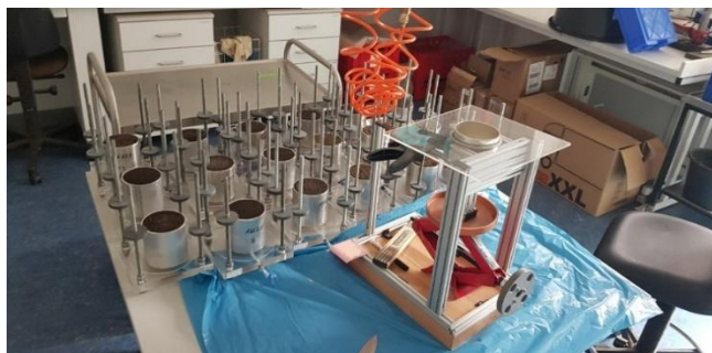
Figure 1: Preparation of soil samples for ^{15}\text{N} gas flux experiments. Manure application via defined above-ground or below-ground application is carried out using the special device in the foreground (source: Balázs Grosz).
