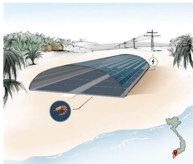
Figure 1: Schematic design of an Aqua-PV-facility with grid connection (Fraunhofer Institute for Solar Energy Systems (ISE), Freiburg, Germany).
