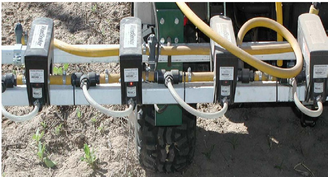
Figure 6.9: Weedseeker™ sensor interfaced to small scale spray boom for weed spraying in bare soil (from McCloskey, 2009).
