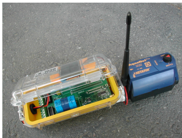
Figure 4.4: A wireless mesh network for remote control of the individual nozzle (personal communication Coates and Delwiche, 2010).
