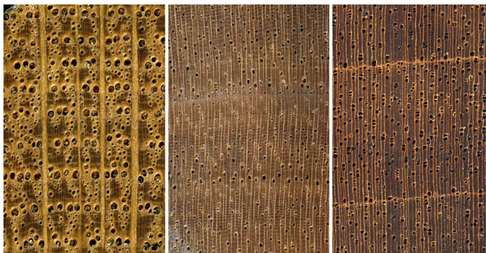
Figure 2: Distribution of vessels in hardwoods. (left): ring-porous structure of oak; (middle): semi-ring-porous structure of walnut, (right): diffuse-porous structure of American mahogany
