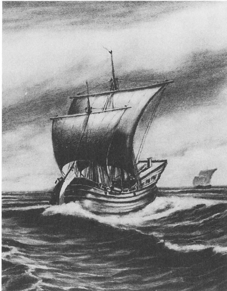
Fig. 15. Typical boat for the herring fishery in the 16th century. This ship served as a freighter as well (maximum load 50 to 60 tonnes) out of the herring fishing season
