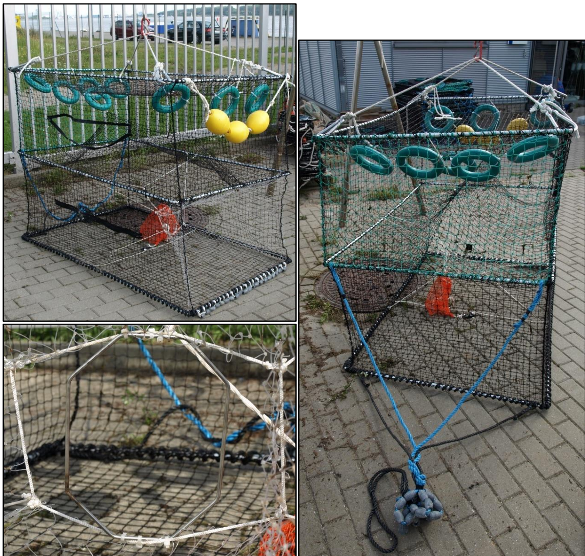
Figure 9: Cod pot-type II was equipped 8 ring floats (0.4 kg buoyancy) and 3 additional floats (0.78 kg buoyancy, yellow, top left picture) to float the pot off the sea bottom. A metal frame in the entrance acted as a seal exclusion device (SED) (bottom left picture). An escape window, consisting of a larger green mesh panel (40 mm square mesh side) was installed in the upper half of the pot. The four-string holdfast was attached on two levels of the pot and equipped with a 4 kg mooring weight (right picture).
