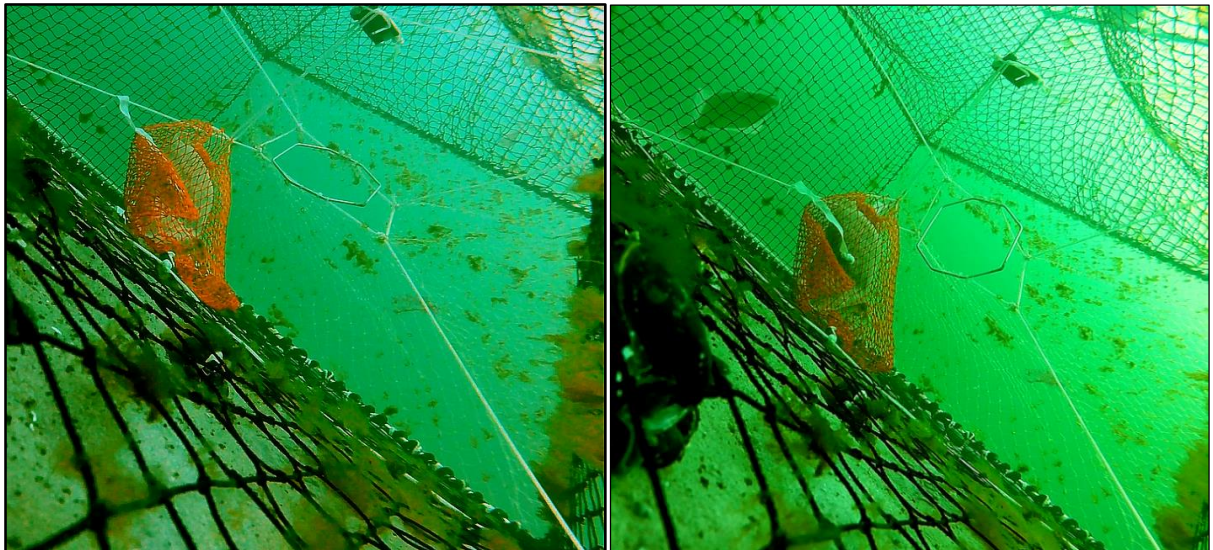
Figure 32: Tilting metal frame SED (left) and flatfish trying to enter the pot (right).
