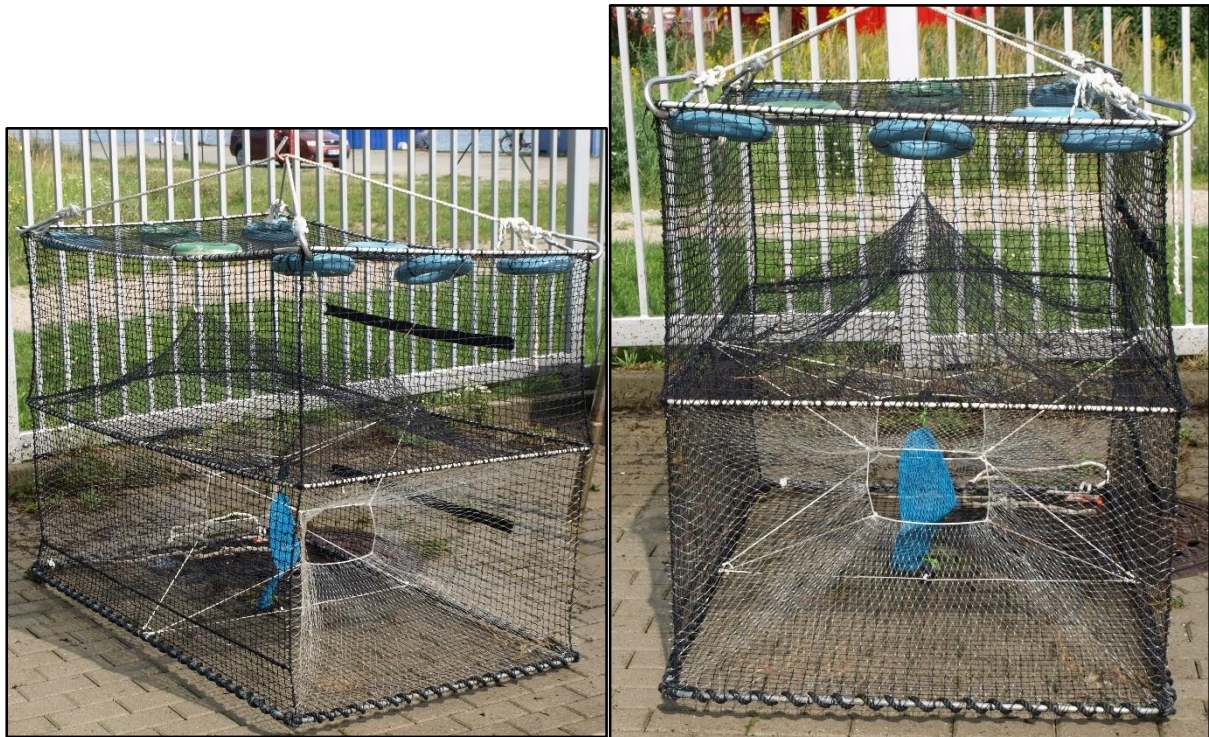
Figure 8: Cod pot-type I. 2 funnel-shaped entrances were facing each other on the short sides of the lower chamber. The lower and upper chamber were separated by a roof-shaped single ply netting with a narrow slit opening. Both chambers could be accessed through horizontal zippers (dark lines in left picture). The blue bait bag was suspended in the middle of the lower chamber. 8 floats (0.4 kg buoyancy) were strapped on the top of the pot to unfold it underwater.
