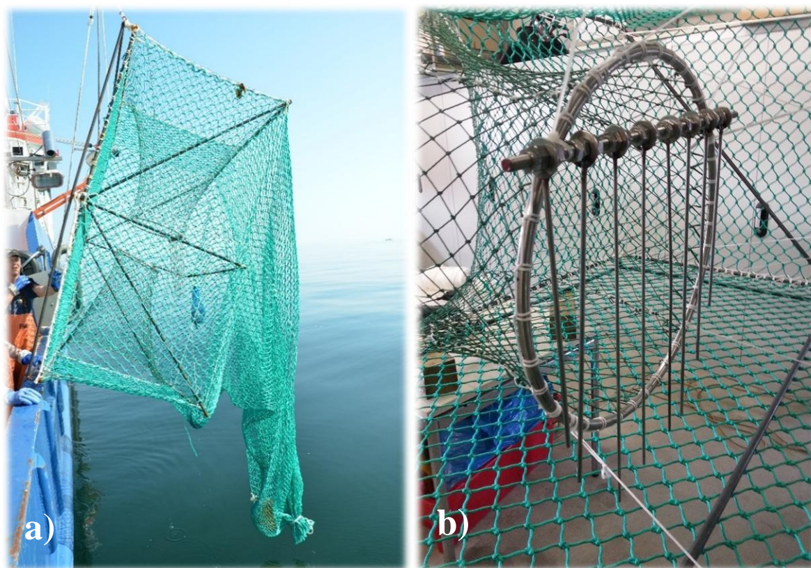
Figure 8: Canadian fish pot. a) Hauling of a pot. b) Trigger mechanism which is implemented in each entrance to avoid escapes.
