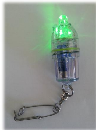
Figure 12: Fishing light type YML-1000 (YM Fishing Corporation) used in fish pots.
