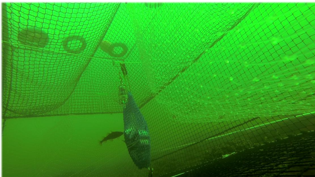
Figure 36: Small cod in Norwegian fish pot with modification 6 (herring, light and entrance) during video observation on 20 th of June 2013.
