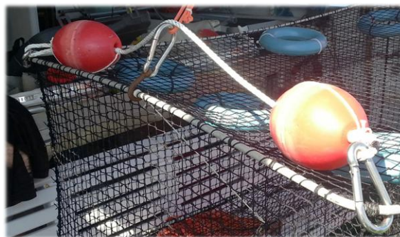
Figure 16: Two additional floats (0.78 kg buoyancy), which were attached to the upper frames on both sides of a fish pot between 24 th of May and 23 rd of June to float them off the bottom.
