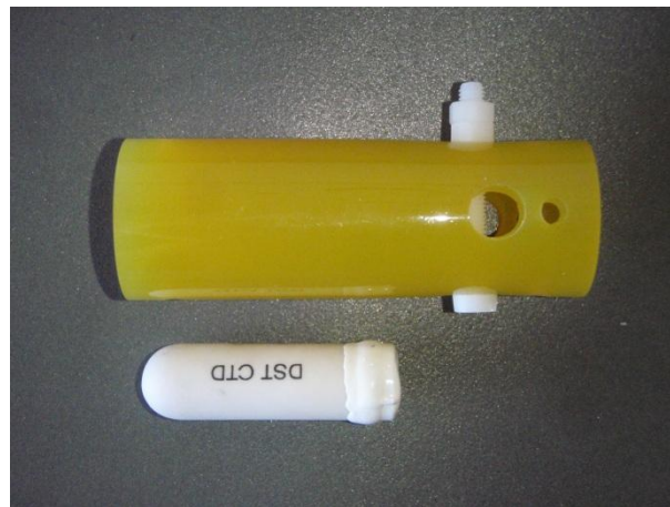
Figure 9: Star Oddi CTD logger and housing. The logger is inserted into the housing before being attached to the beam. The screw ensures that the logger does not fall out. A cable tie is also fastened for security.
