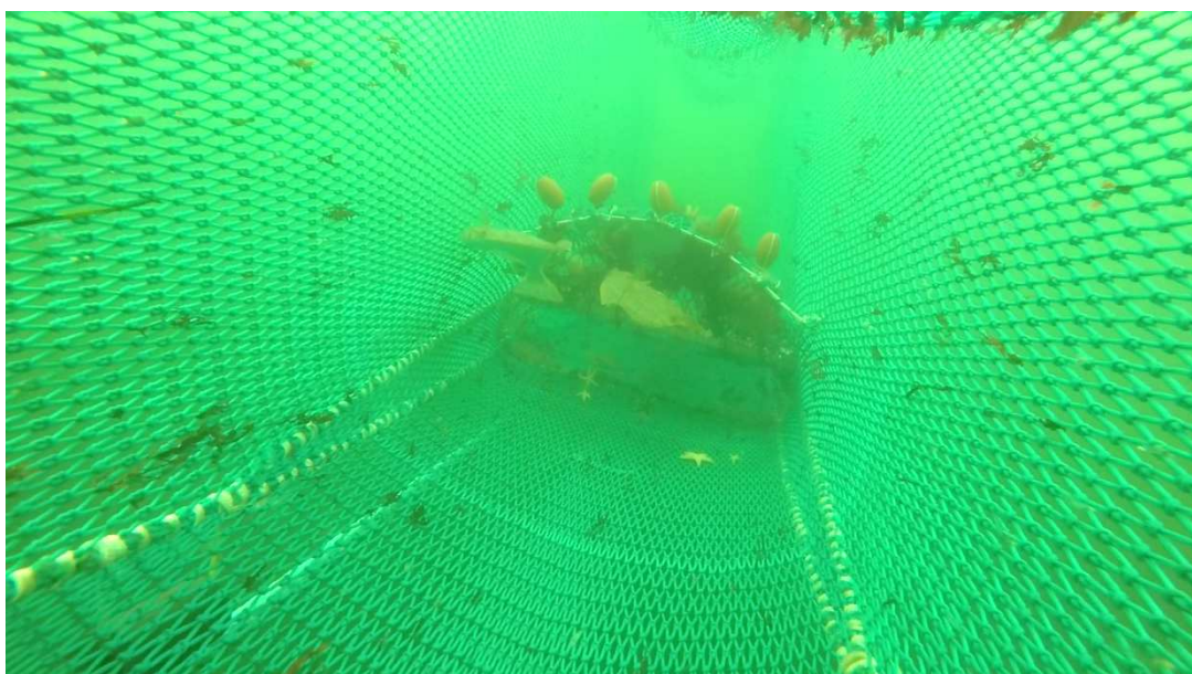
Figure 25: Screenshot of underwater video recording. Shows flatfish staying near the trawl bottom. (haul 7, during reeling)
