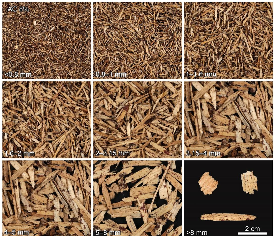
**Figure 2.** Sieve-fractionated Particle Material 2 (AC 8%).
