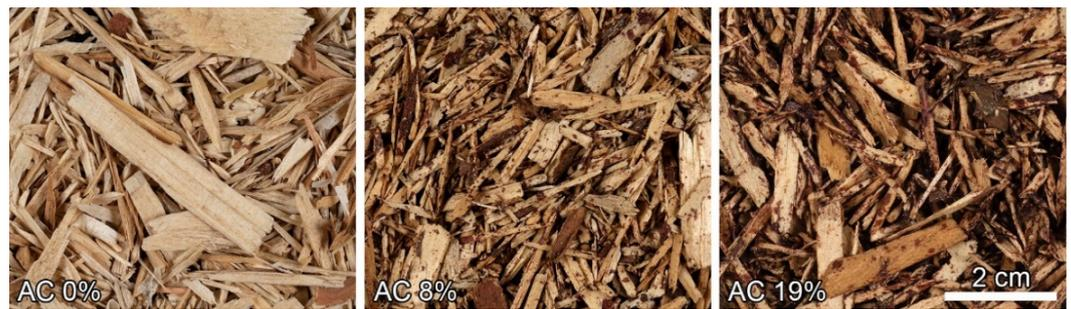
**Figure 1.** Particle materials (PM) of different adhesive content (AC): PM 1 (AC 0%), PM 2 (AC 8%), PM 3 (AC 19%).
