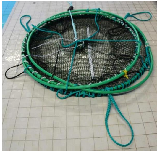
Fig 1: Fish cages used for exposure experiments with the flatfish species common dab ( L. limanda ) in munitions dumpsites in shallow waters (10-15 m) of the western Baltic Sea (photos: T. Lang, Thünen-Institut)
