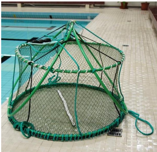
Fig 1: Fish cages used for exposure experiments with the flatfish species common dab ( L. limanda ) in munitions dumpsites in shallow waters (10-15 m) of the western Baltic Sea (photos: T. Lang, Thünen-Institut)
