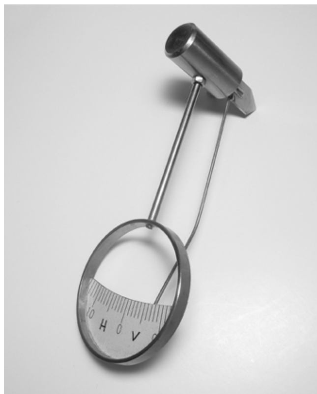
Figure 1. – Measurement device for measuring grain angle of standing trees. On the measurement scale “H” and “V” indicate right-handed and left-handed spiral grain, respectively.
