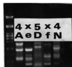
Figure 4. – Agarose-gel electrophoresis of the fragments obtained by PCR amplification of hybrid (xe and xf) and parental (4A and 4N) genomic DNAs with OPN06 primer. (4A). P. alba , (xe) P. deltooides x P. alba 7/32B, (5D) P. deltooides , (xf) P. euroamericana ( P. deltooides x P. nigra ) I-214 and (4N) P. nigra .
