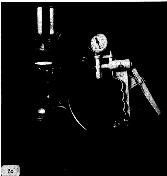
e) Filtrate passed through a 3 \mu Milipore filtration system, pollen deposited on filter.
