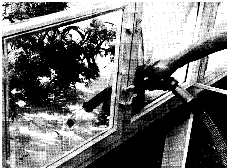
Fig. 5. — Pollen from oak catkins is sucked up from the cellophane by means of a vacuum cleaner (cf. description page 3 and diagram fig. 6). The mouthpiece is operated through a plastic funnel to prevent contamination by foreign pollen.
