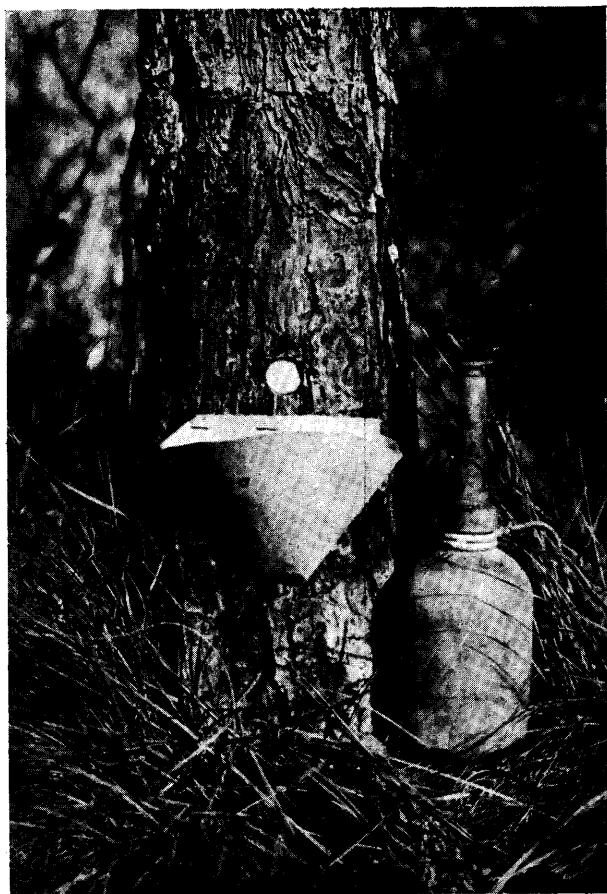
Fig. 2. — Micro-tapping technique used to collect gum samples in longleaf plantation. A \frac{3}{4} -inch bark patch is lifted out with a metal punch and the wound is sprayed with 50-percent sulfuric acid to prolong the gum flow. Gum collects in the paper cup.
