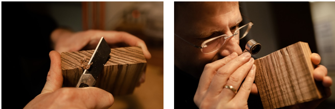
Fig. 1. Preparation of the transverse plane and macroscopic observation / identification of the timber
