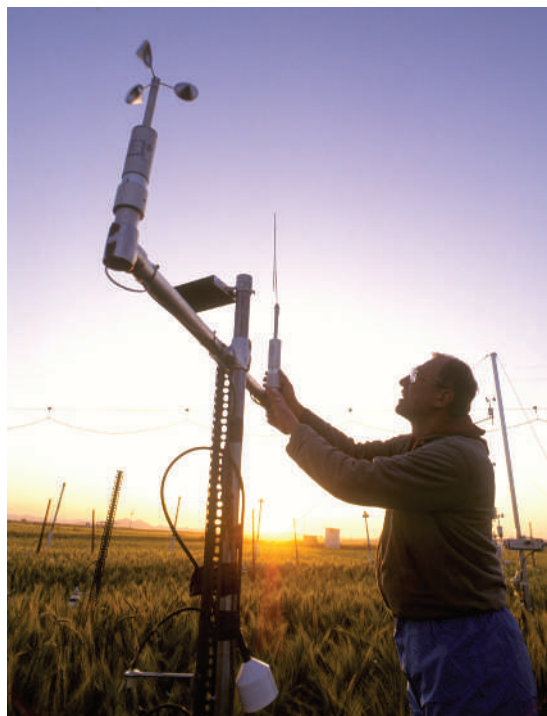
Feedback from wind sensors helped Bruce Kimball control the release of CO 2 in a FACE study on wheat.
