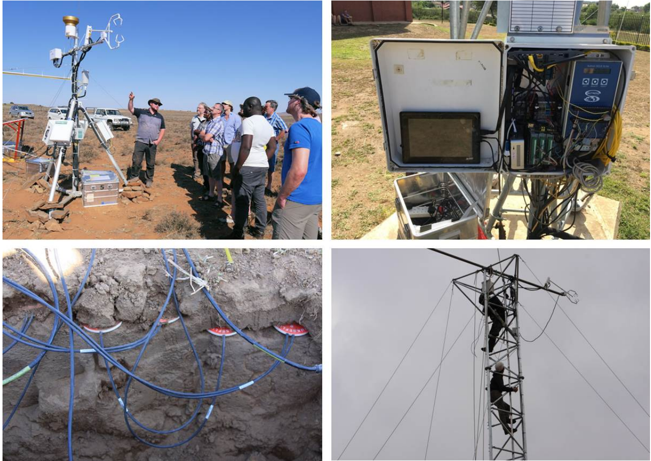
Figure 1.2: Introduction of the Karoo tower infrastructure to the ARS AfricaE consortium by TI-AK engineer J.-P. Delorme (top left); installation of soil heat flux plates (bottom left); close-up of Vuwani Biomet system (top right); working up in the Vuwani tower (bottom right).
