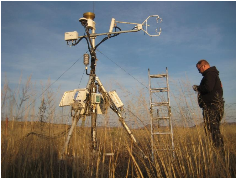
Fig. 3 Maintenance of a greenhouse gas measurement tower in The Karoo, South Africa © Thünen Institute AK, J.Ch. Jüdt
