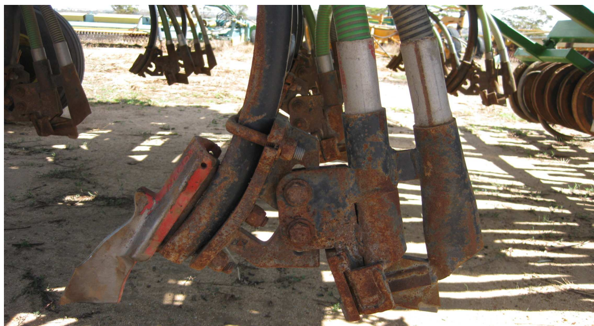
Figure 4.5: Tine seeding unit implemented on AU 4000WB
