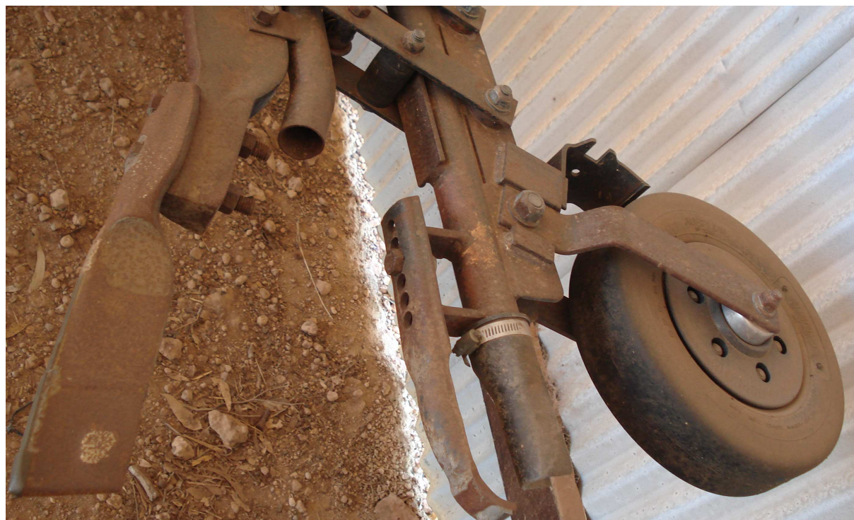
Figure 4.6: Tine seeding unit implemented on AU 2800CW
