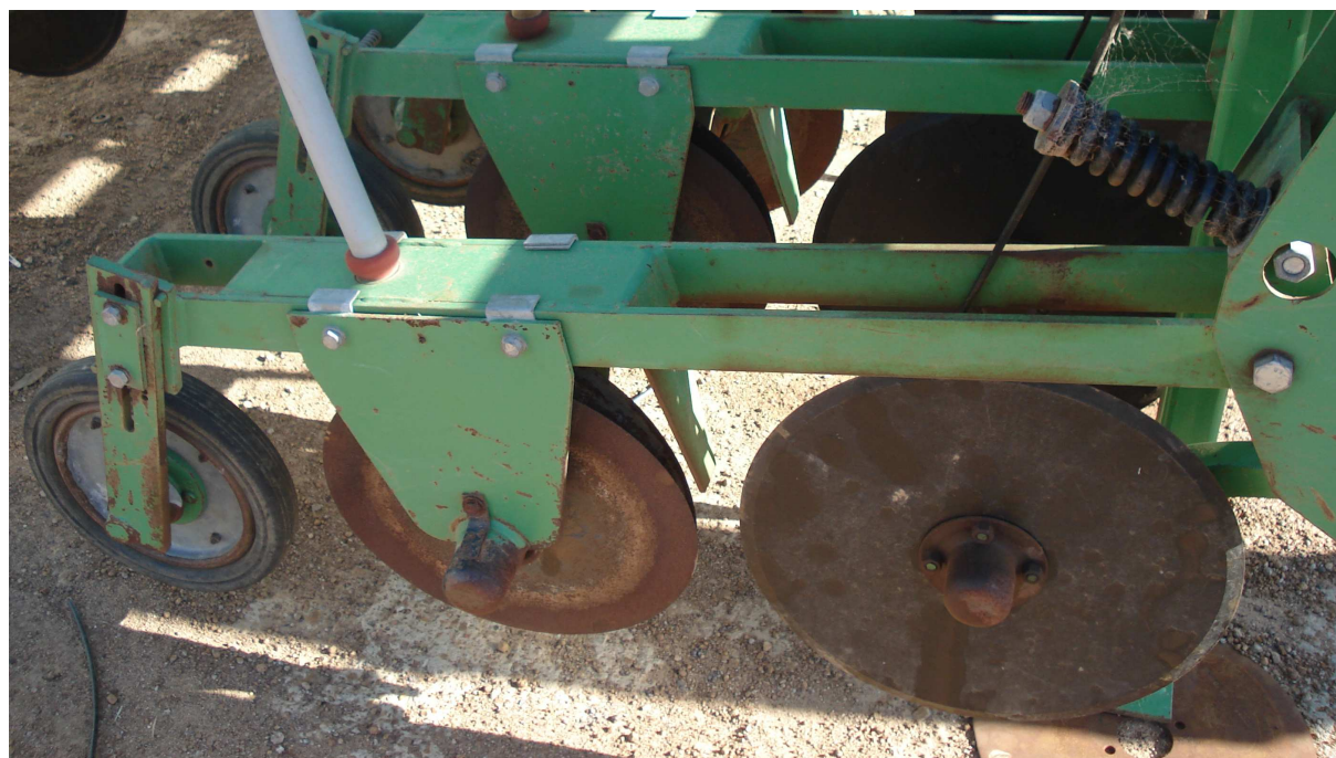
Figure 4.3: Disc seeding unit implemented on AU 4500SC
